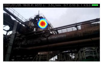
The compressed air leak from the pipe in high place out of reach is found.
